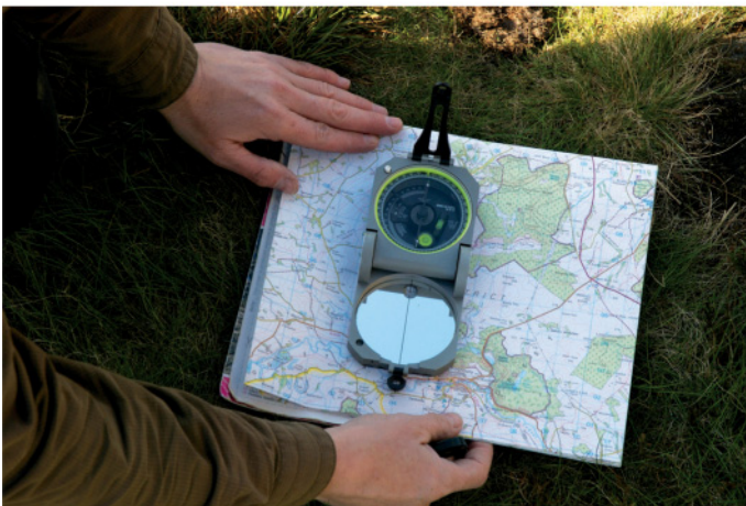
Figure 2.11 Triangulation using a Brunton-type compass. The terms for the different parts of the compass-clinometer are given in Figure 2.3a–c. (Map: Ordnance Survey, Landranger Series, Sheet 81. Ordnance Survey on behalf of HMSO © Crown Copyright 2010. All rights reserved. Ordnance Survey Licence number 100018362. (extract is from within 10 km grid square NU(46)00.)
