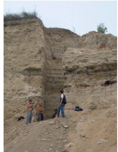
Figure 5.9 Example of a trench through diatomite in China. Successive samples were obtained as the trench was dug. (Robert A. Spicer, The Open University, UK.)
