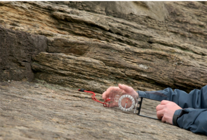
Figure 2.6 How to use the Silva-type compass-clinometer to measure the orientation and dip of a plane using the contact method. The parts of the compass-clinometer are shown in Figure 2.3d and e.
