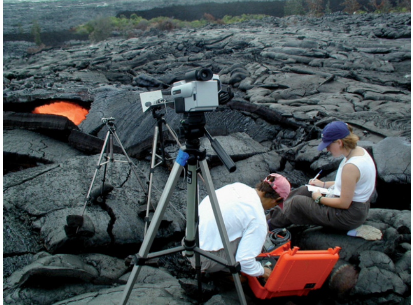
Figure 7.24 Two infrared thermometers and one infrared video camera have been set up to look into this skylight on an inflating pahoehoe field, to record variations in the rate of flow in a lava tube on Kilauea, Hawaii. (David A. Rothery, The Open University, UK.)
