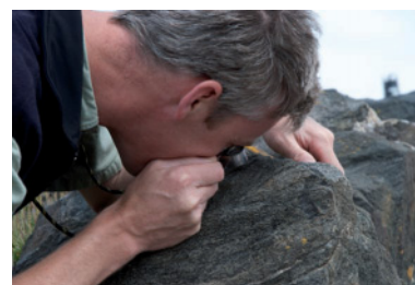
Figure 2.2 Photograph to show correct use of the hand lens. Note that the person is holding the lens close to his eye. The lens is fastened on a lanyard around his neck for ease of access and use.
