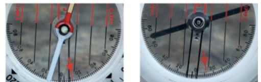
Figure 2.6 How to use the Silva-type compass-clinometer to measure the orientation and dip of a plane using the contact method. The parts of the compass-clinometer are shown in Figure 2.3d and e.
